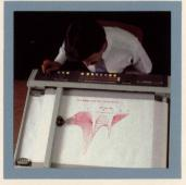
Simplified graphic data input (top). The 4956 Graphic Tablet inputs graphic data to the 4054 directly from engineering and scientific drawings, from schematics or layouts via a digitizing pen (shown above) or cursor.
