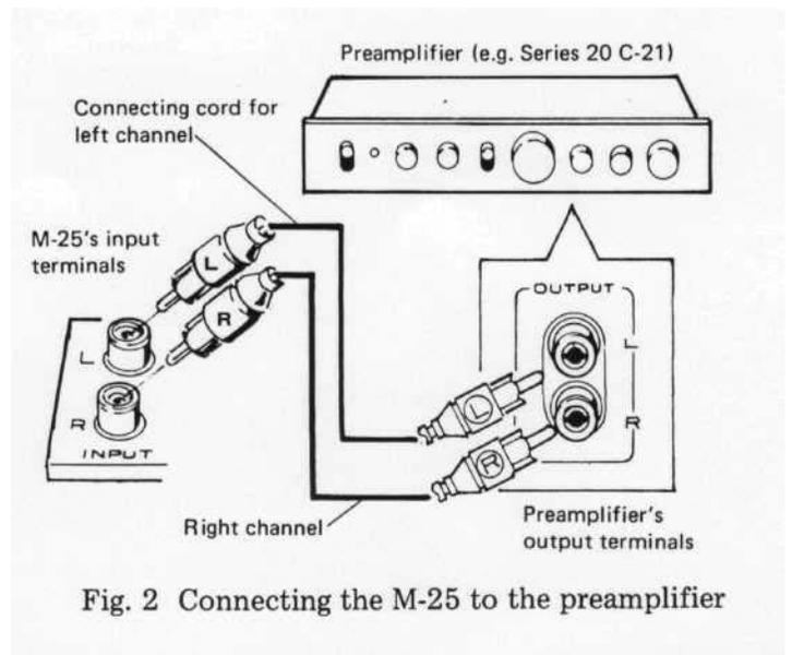
Fig. 2 Connecting the M-25 to the preamplifier
