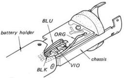
2) Unsolder four lead wires at circuit board.
