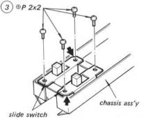
Cut corner of slide switches should be placed as shown by arrow.
