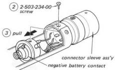
4 Unsolder four lead wires at negative battery contact.
