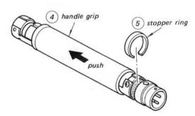
Note: When remove the handle grip, do not touch diaphragm of capsule.
