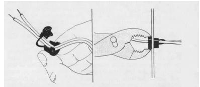
25() Separate the two conductors of the line cord from the stripped end to the strain relief, and cut off 9 1/2" (24 cm) from *one* (either) conductor. Strip about 3/8" (1 cm) of insulation from the short-cut conductor, and connect it to power fuse holder lug #2 (S). Position the other (long) conductor against the chassis on the left side. This conductor will be connected later.
