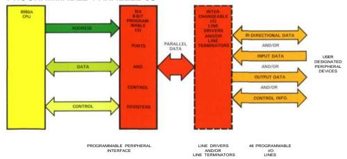
The SBC 80/10 programmable parallel I/O interface provides the capability of using the system program to configure the direction and mode of information flow between user designated peripheral devices and the six 8-bit I/O ports on the SBC 80/10.
