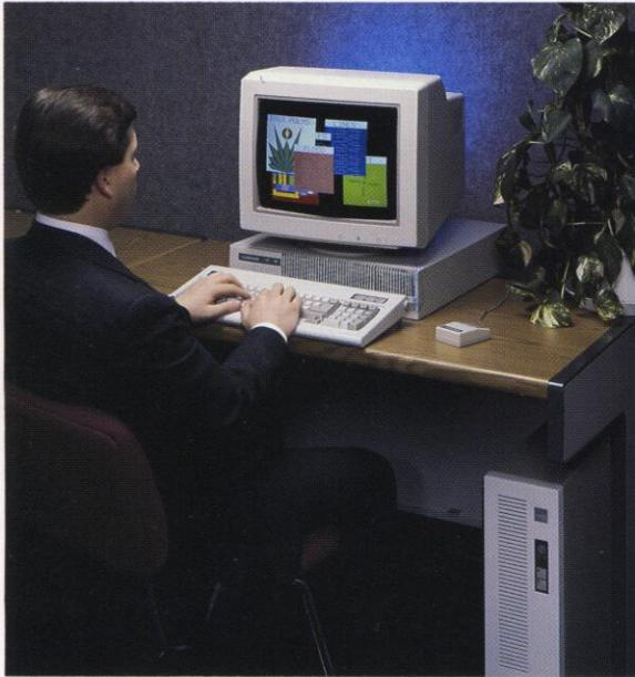
The combination of the high-performance PG 90 graphics display system and IBM's Personal Computer AT creates a powerful graphics workstation.
