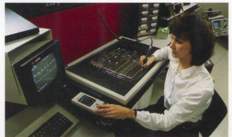
All printed circuit boards are tested using GenRad's 2272 in-circuit tester.
